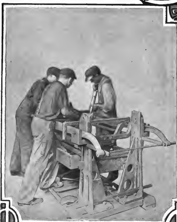
F—Special Jigging Fixture Designed for Use in Assembling Chassis Frames, so Contrived That All the Holes Are Drilled Interchangeably and the Work Is Held Securely in Position During the Process of Riveting
